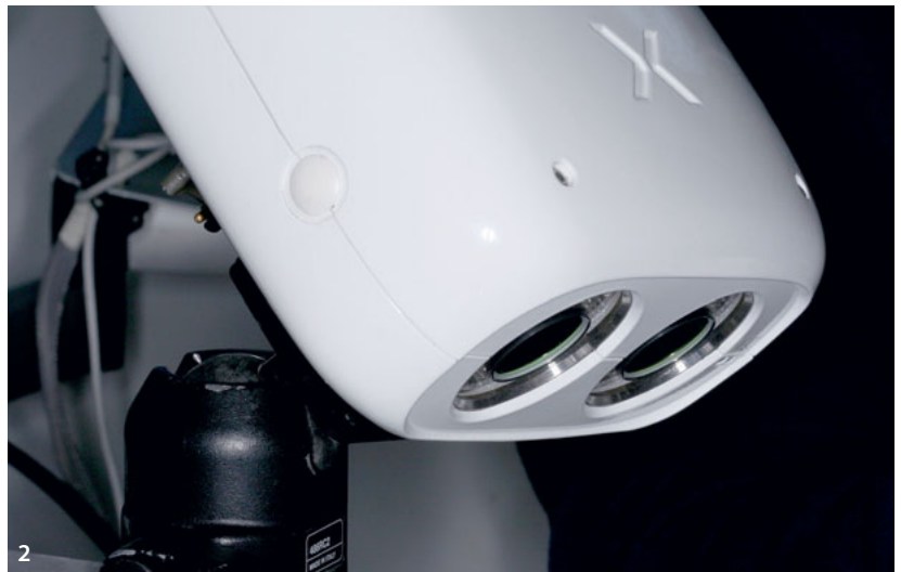
Fig 2 PICcamera. This stereocamera identifies the PICabutment in its 3D position.
